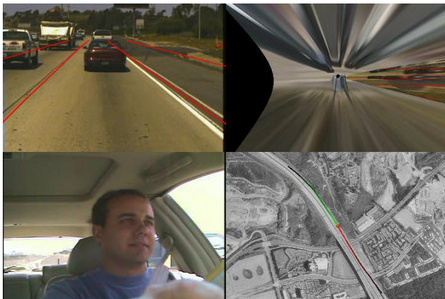
Figure 4 Video post-processing showing the video streams synchronized with GPS information and an aerial map as well as a local map constructed from the surround videos
