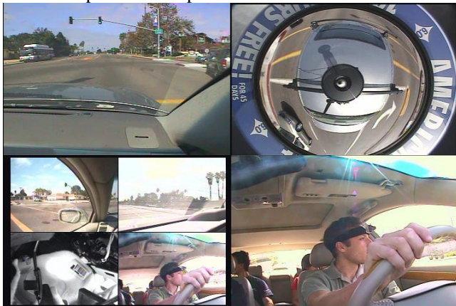
Figure 3 Video streams collected by the LISA-Q capture system
